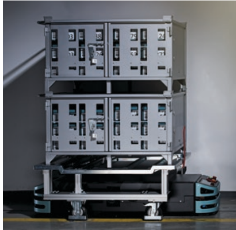
Top: Each NotaTracc tray has a unique identification number, which can be read by a barcode or RFID reader. A transparent cover and a seal ensure the necessary security.
