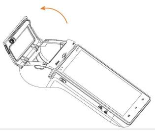
Fully open the printer cover and remove the old roll of paper; Carefully place the paper roll into the printer compartment. Close the printer cover carefully and push firmly until it locks.
